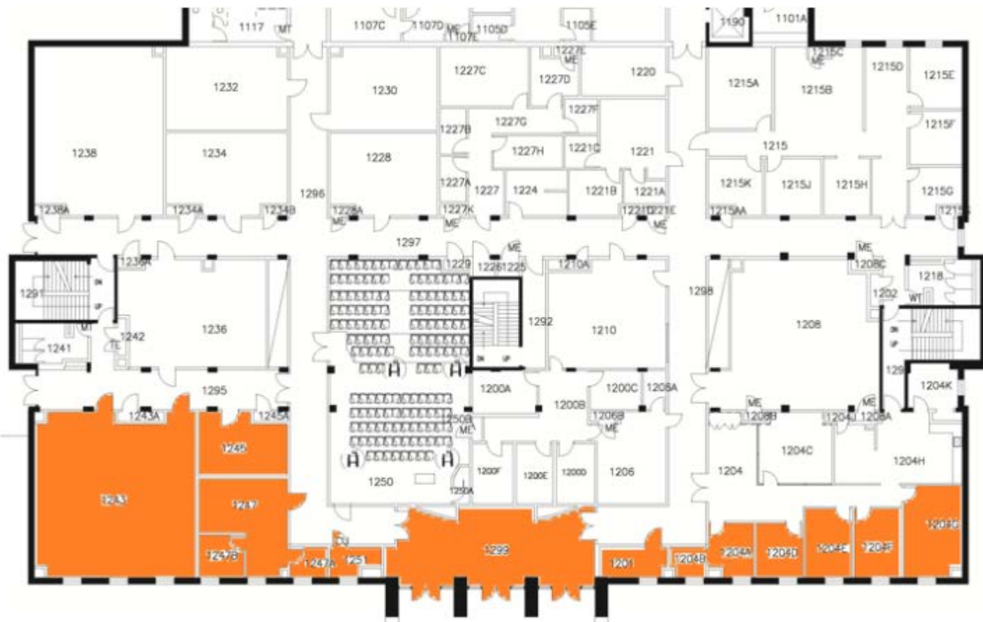
Map of impacted areas of the HVAC Heating outage on the first floor, Wing 2 of the BPS Building
